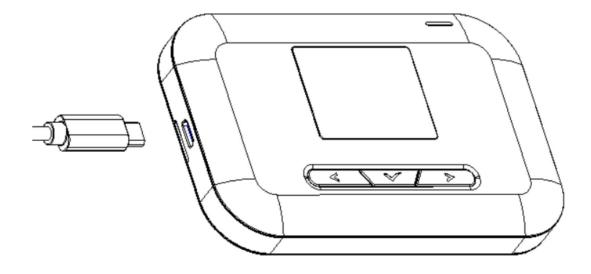
2. The indicator light on the power button illuminates red when charging starts. It may take up to three hours to fully charge the battery. The light will turn green when the device is fully charged.
